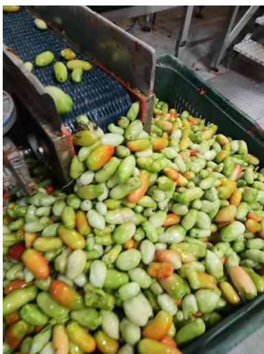
Fig. 1 Green unripe tomatoes: manual and optical sorted at La Torrente Industrial Tomato Plant
